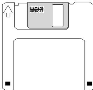
Hold the disk so that the arrow symbol is at the top and points away from you. Now insert the disk in the drive slot provided. The disk has been correctly inserted if the gray ejection button has popped out.
