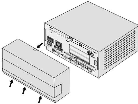
In order to mount the cable cover, insert it in the guides marked with arrows in the figure below. In doing so, ensure that the cable cover does not fit askew.
