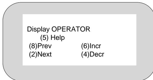
If an internal CRT-adaptor is plugged in you can see the following screen mask. For the settings LOW and MIDDLE the system memory will allocate 1,5 MB for the graphical section. In the setting HIGH it will allocate 2,5 MB.
