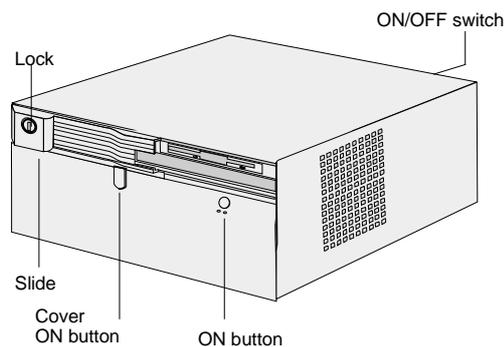
You can now switch on the BEETLE /M by means of the switch on the rear of the housing and push the ON button at the front for a short time. You may have to unlock the slide and move it to the left.
