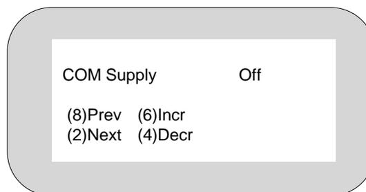
With “COM Supply On” the CPU switches from sleep mode to standard mode when one of the following interrupts is actuated: IRQ1 (keyboard), IRQ3 (COM2), IRQ4 (COM1), or IRQ8 (RTC).
