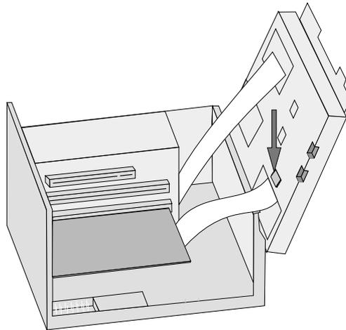
Then flap the carrier back so that you can install the new hard disk. Just put it on the guide rail and push it back until it snaps in. Plug in the connectors again.
