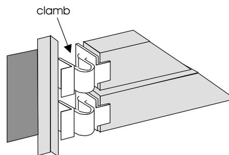
First check whether the jumpers (if present) of the card are set correctly to avoid internal system conflicts. The correct setting for the jumpers can be found in the documentation for the plug-in card. Then slide the expansion card into the slot provided. Ensure that the card establishes contact with the terminal strip.
