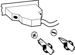
The interface connectors screws made of metal can be secured with a screwdriver. Screws made of plastic must be secured manually only.
