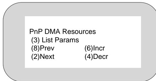
This mask only works together with an operating system that is capable of Plug-and-Play (PnP) functions. Setting "Yes" has the effect that the BIOS will initialize only those components necessary for booting the operating system. All the other PnP components must then be configured by the loaded operating system.
