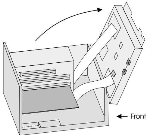
Remove the respective metal cover at the backside of your BEETLE/M by removing the screws with a socket wrench. Then bring the socket through the recess of the housing and plug in the card (see drawing). Attach the socket using the screws that you removed before.
