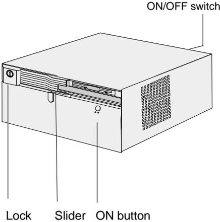
The ON button can be protected from access using the lockable slide.
