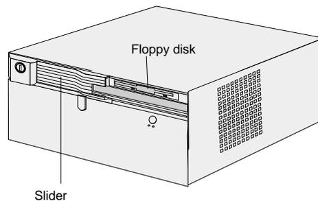
The lockable slider can be used to prevent unauthorized access to the disk drive.
