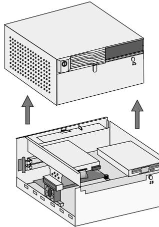
Lift up the carrier of the hard disk and the floppy disk drive by loosening the knurled screw (see drawing) manually or with a screwdriver. Then pull the carrier forward to the stop and lift it up to the front side.
